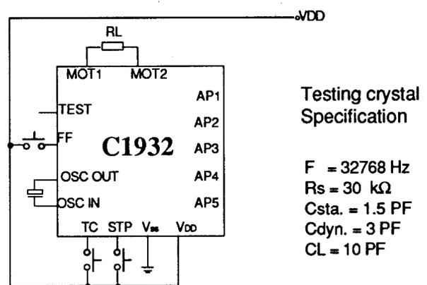
Note: Substrate should be either left open or connected to VDD
