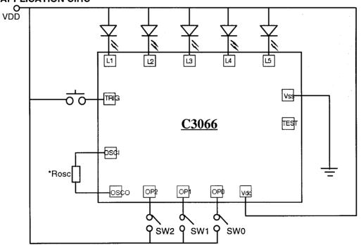
Note: Substrate must be connected to Vss.
