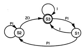
At S3, the time pulse counter N is reset and counts. Overflow signal I is generated when N counts full. S3 is maintained until PI is detected which switches the division cycle to S1.
