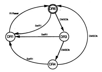
In DR6, R6 is displayed on the right 2 digits with the left 2 digits blanked. In DR3, R3 is displayed with a decimal point between the 1 st and the 2 nd digits from the right, blank leading zero of up to 2 digits is provided. In DR4, the least 4 digits of R4 is displayed without blank leading zero. Three display mode flags indicating mode status are provided.
