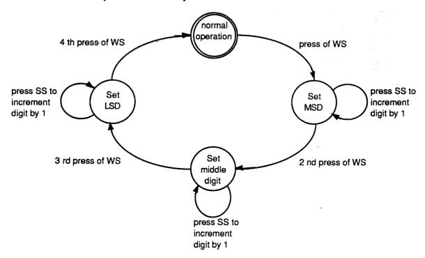
Upon the 1 st press of WS, the counter constant (content of R1) will be displayed on the right most 3 digits of the LCD panel with the most significant digit flashing once every second. The flashing digit will increment by 1 for each press and release of SS.
