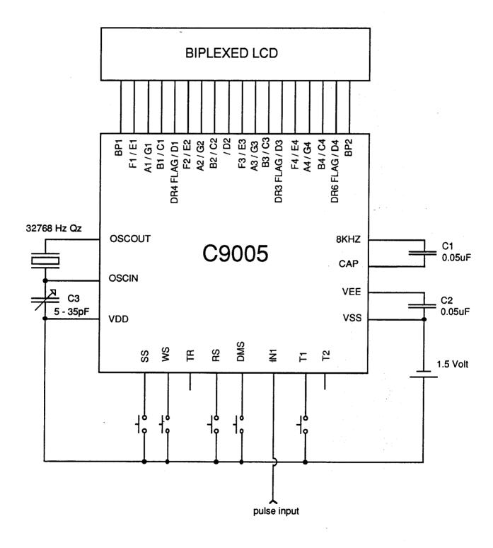
TR - option input for testing, connect it to VSS will force the device to power-up reset. T2 - option input for testing.
